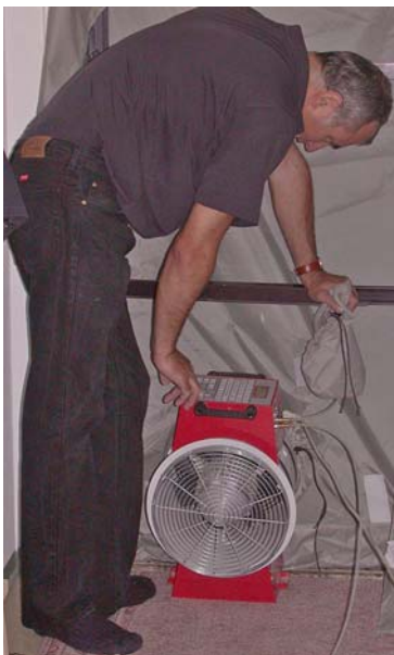
Figure 3.17 and 3.18 Testing the airtightness of a wall during the construction stage (left) in order to verify airtightness. Air leaks are traced e.g. with smoke and anemometer measurements (right)
